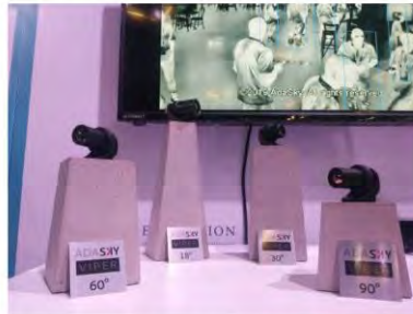
AdaSky's Viper cameras use far infrared sensors to create a more accurate picture for autonomous vehicles. AdaSky
