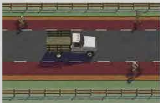
Figure x-x. Motorists travel in the center two-way travel lane. When passing a bicyclist, no lane changes necessary.
